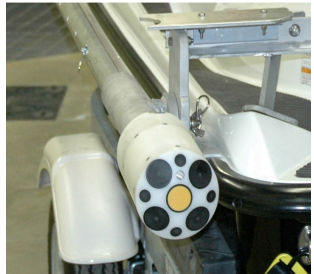
The Jag Ski is nimble, fast and cool - and outfitted with a full suite of water quality sampling and water velocity equipment, such as the SonTek RiverSurveyor M9 multi-frequency system you see here.
