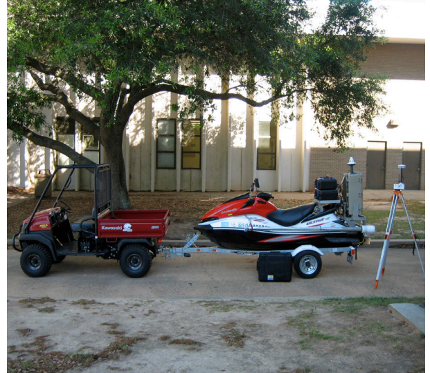
The South Alabama Jag Ski and 4x4 towing vehicle and SonTek RTK GPS solution, which offers an incredibly precise, fully integrated boat speed solution to augment, or be an alternative to, bottom tracking.
