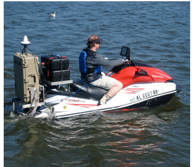
Bret Webb has used his Jag Ski - outfitted with a SonTek acoustic Doppler Profiler (RiverSurveyor M9) and a Portable Sea Keeper water quality testing system - for bathymetric surveys, multi-parameter water quality testing, and studies of the flow of water and pollutants in the Mobile Bay estuary system.
